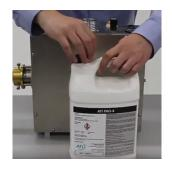
**CAUTION:** Paraffin Oil and Corn Oil should NEVER be used as reagents for Thermal Aerosol Generators.
