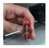
**Step 4.** Inspect fuses to see if they are blown. Replace fuses as needed according to the table below.
