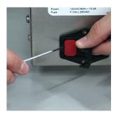
Step 3. Remove fuse holder using a flat-head screwdriver.
