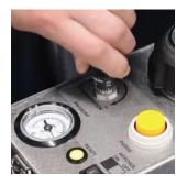
**Step 7.** Turn metering valve two turns counter clockwise to start flow. Unit will produce aerosol in about 10 seconds. Once started, adjust as needed.
